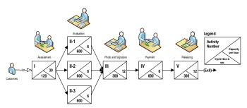
Figure 6. Process Flow Diagram with Cycle Time and C apacity
