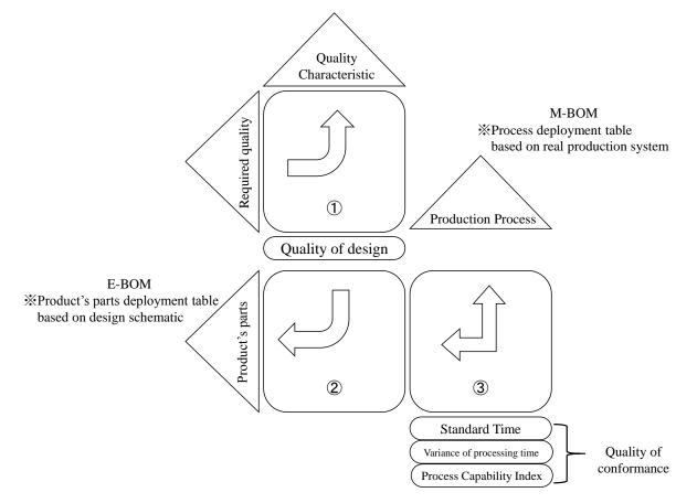
Figure 6: Conceptual design of QFD considering production efficiency
