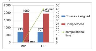
Figure 2: Measurement of performance between MIP and CP when solving objective 1
