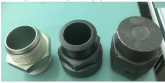
Figure 2: Product photos (cold forging, hot forging).
