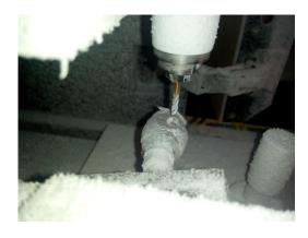
Figure 14: Dirty and dusty environment due to resin chip.
