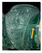
Figure 12: Crack due to over clamped
