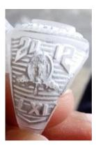
Figure 13: Machining result with resin as material
