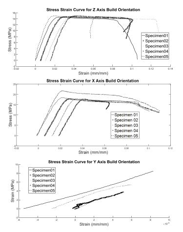
Figure 4: Engineering Stress Strain Curves for Z-ABS Material for X, Y, Z Orientations (from top) Respectively
