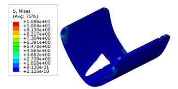
Figure 9: FEA Results for Limb Attachment (After
