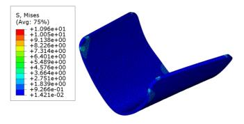
Figure 8: FEA Results for Limb Attachment (Before Optimization)
