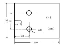
Figure 3: Geometry of the specimen
