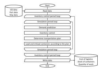
Figure 5: Procedures of marine logistics simulator
