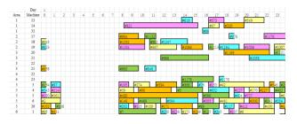
Figure 7: The Gantt chart of filling process.
