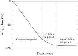
Figure 6 Sludge drying time curve
