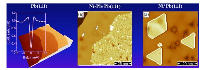
Figure: Superconducting gap measured at the pristine Pb(111) substrate (Left). STM topography of monatomic Ni-Pb surface alloy on Pb(111) by means of high temperature growth (Middle). In contrast, honeycomb-structured Ni nanoislands can be fabricated on Pb(111) by low temperature deposition (Right).
