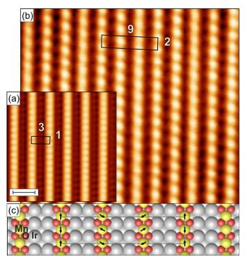
Figure: Atomic resolution scans of  $MnO_2$  chains on Ir(001). (a) A (3 × 1) structural unit cell is observed with a non-magnetic W tip (scale bar: 1 nm). (b) With a Cr-coated W tip the magnetic (9 × 2) unit cell is resolved. (c) Schematic model of the chiral (9 × 2) spin structure of MnO<sub>2</sub>/Ir(001).
