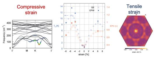
Figure: Calculation results in Li-intercalated bilayer  $MoS_2$  (Left) electron-phonon interaction projected on phonon band structure under 5.5% compressive strain (Middle)  $T_c$  as a function of strain (Right) nesting function under 6% tensile strain.
