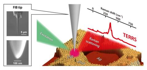
Resolving the Correlation between Tip-Enhanced Resonance Raman Scattering and Local Electronic States of ultrathin zinc oxide films with 1 nm Resolution [2].
